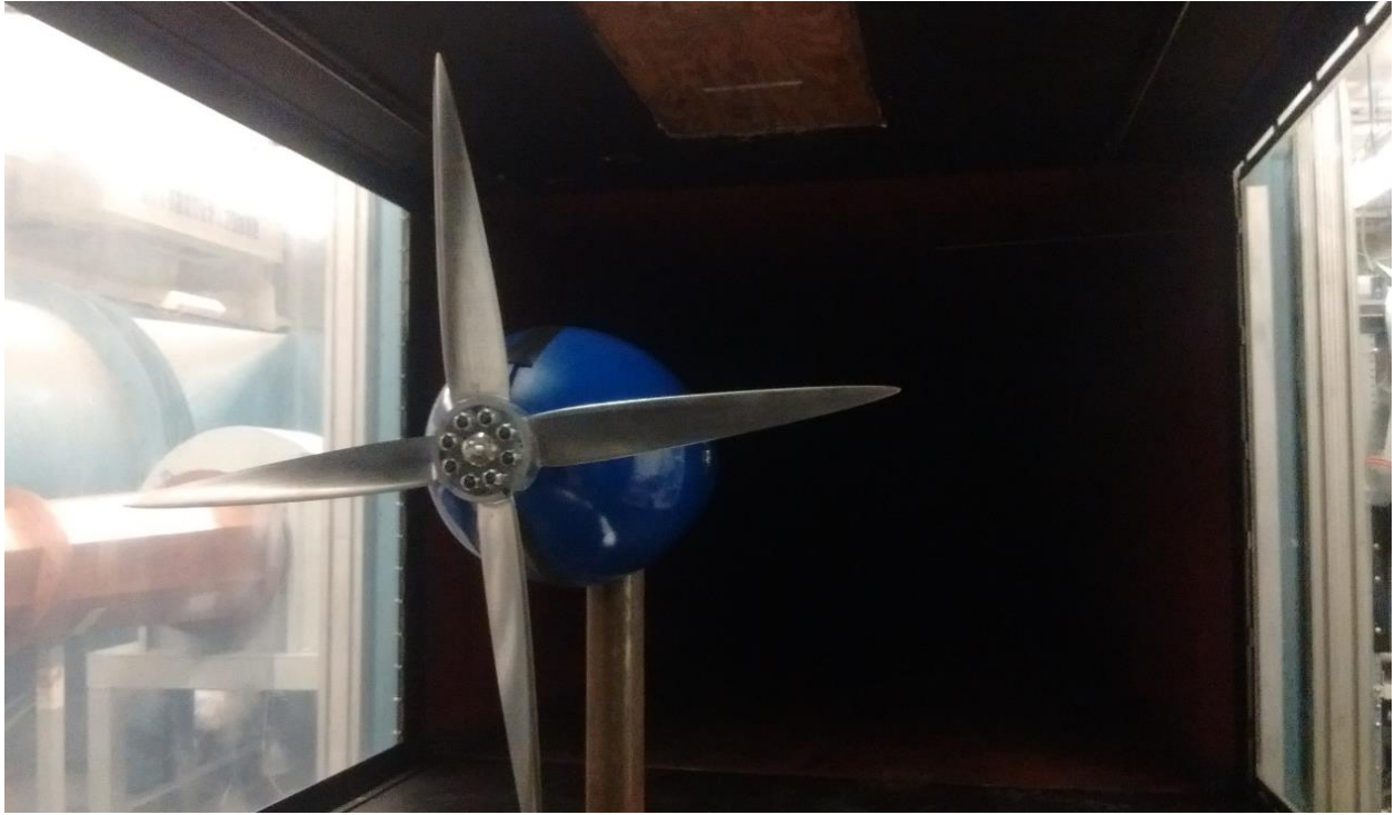
Figure 15- Propeller test stand mounted in wind tunnel with Georgia Tech propeller installed
